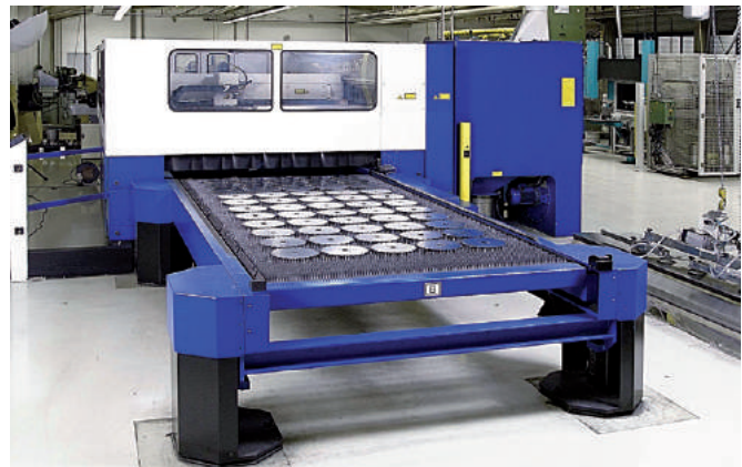
Feinrichten · High-precision straightening of the blades
