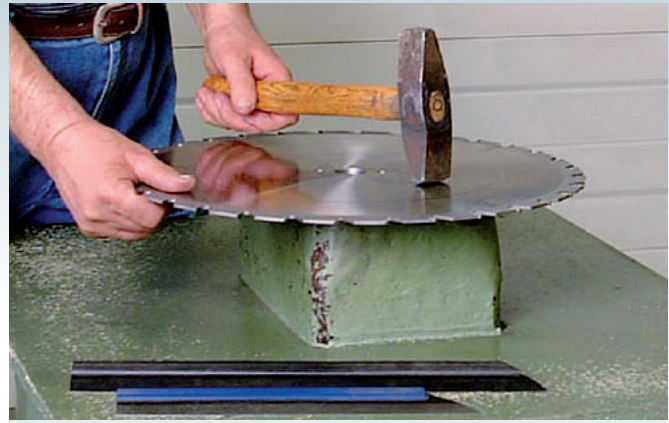
Feinrichten · High-precision straightening of the blades
